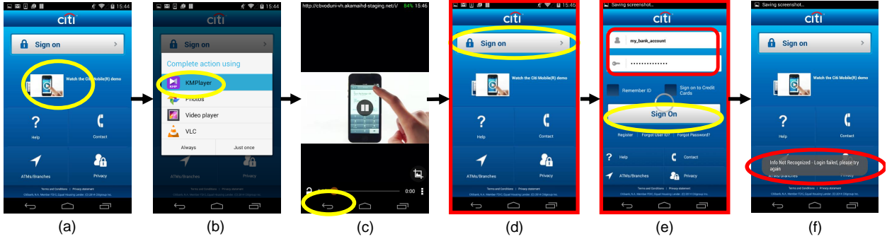
Figure 5: “Back Hijacking” phishing attack to a well-known bank app. (a) the main activity of the bank app, with a tutorial video link for new users; (b) A system dialog showing available video players after clicking the video link; (c) video player activity, user clicks “back” button to quit the video and “goes back” to the original main activity; (d)-(e) the back button directs the user to the phishing UIs, which steal users’ bank account information, then quit after user clicks “Sign On”; (f) The original main activity is resumed, with a log-in failure error message left by the malware on screen.
